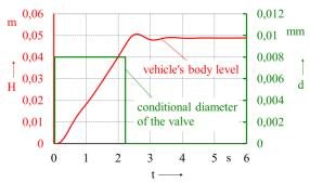
Fig. 11. The working process of setting the target level of the vehicle body with one control action on the solenoid valve
