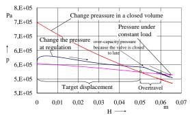
Fig. 8. Illustration of the working process of controlling the level of the vehicle body when over-adjusting the pressure
