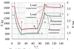
Fig. 6. Verification of the pneumatic spring model
