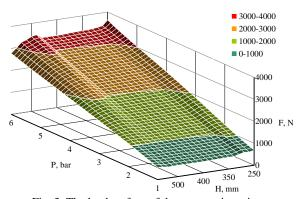
Fig. 3. The load surface of the pneumatic spring
