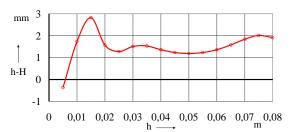
Fig. 12. The accuracy of setting the target level of the motor vehicle body by the regulator according to system (5)
