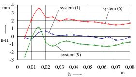
Fig. 13. Comparison of the accuracy of setting the level of the motor vehicle body by the considered regulators
